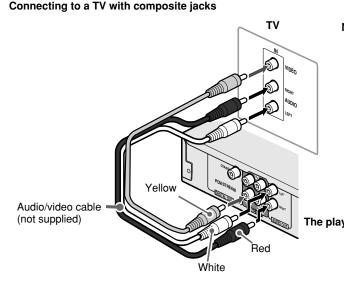
The VIDEO jack, AV OUT terminal, and component (Y, PB, PR) jacks cannot be used at the same time.
